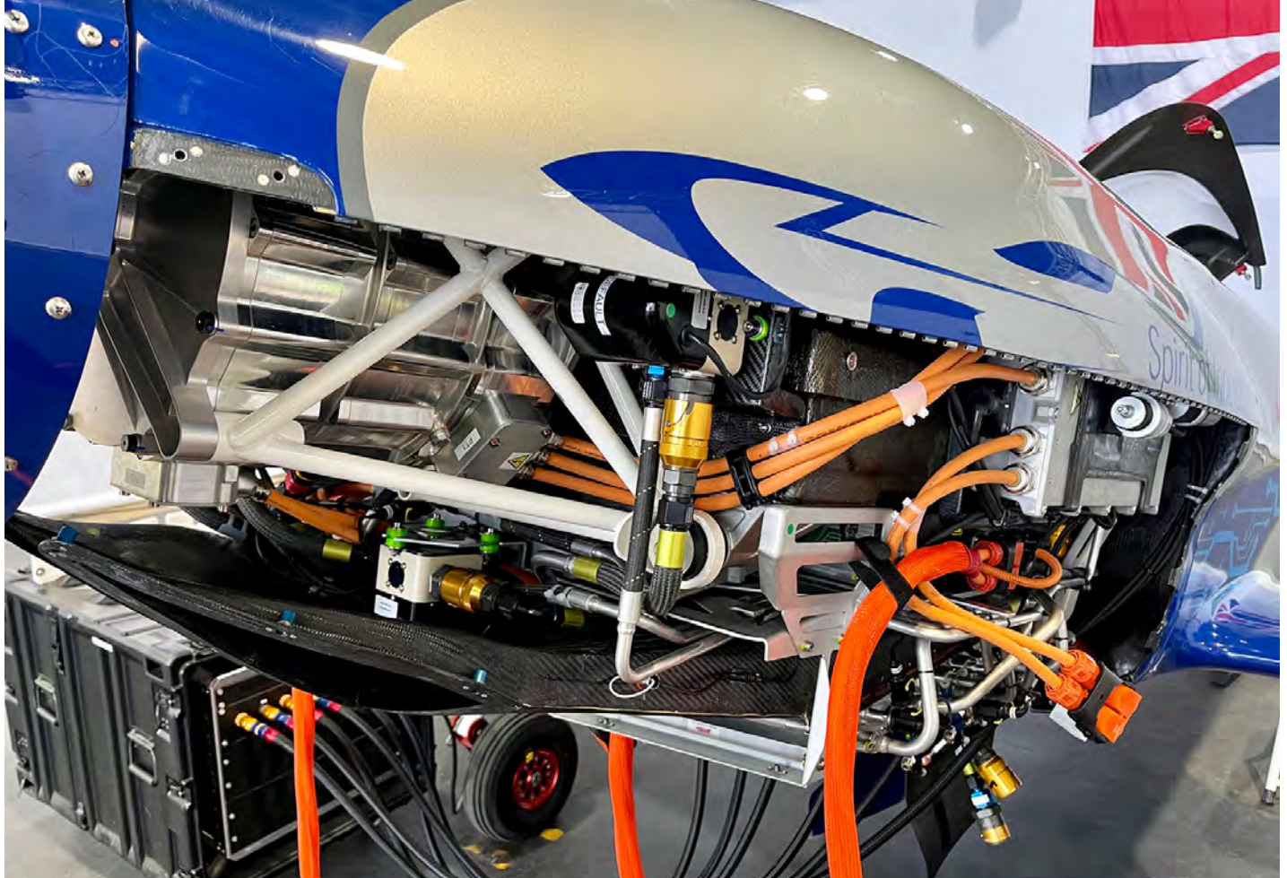
Above Close up of the Propulsion system on charge, lower cowling removed Below Very visual electronic checklist format used across all aircraft flown by the Rolls-Royce operations team, all key checks, speeds and emergencies are covered
