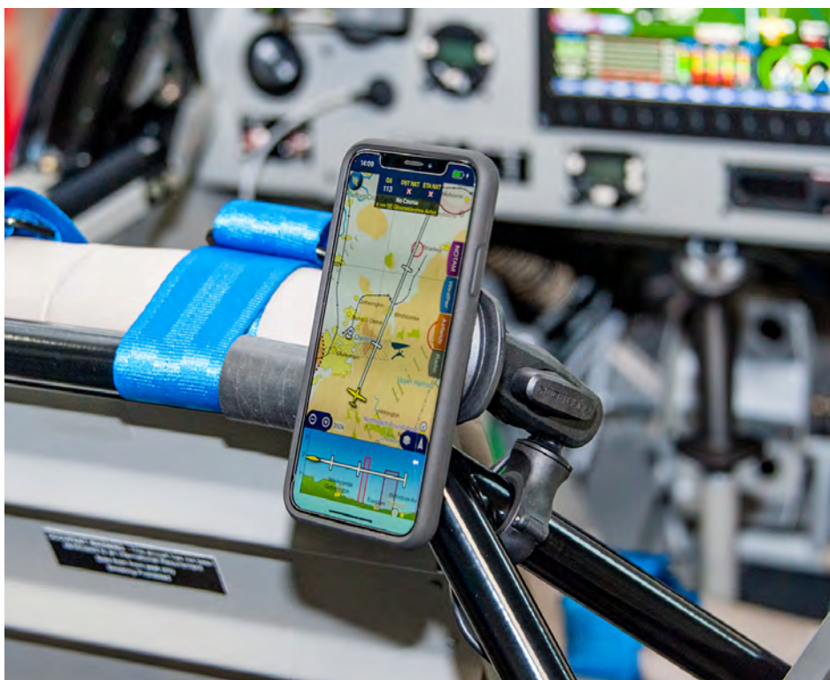
Above The Quad Lock fix for providing some navigation information for the RV-8's backseat passenger. A USB power lead runs up the back of the black tubular support frame to provide power for the charger
