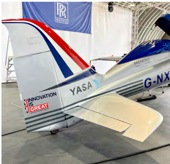
Above Low area high aspect ratio wings are key to the NXT performance Left Fin extensions added to NXT over time to increase stability Below Thread in between tape lines to help with directional stability control
