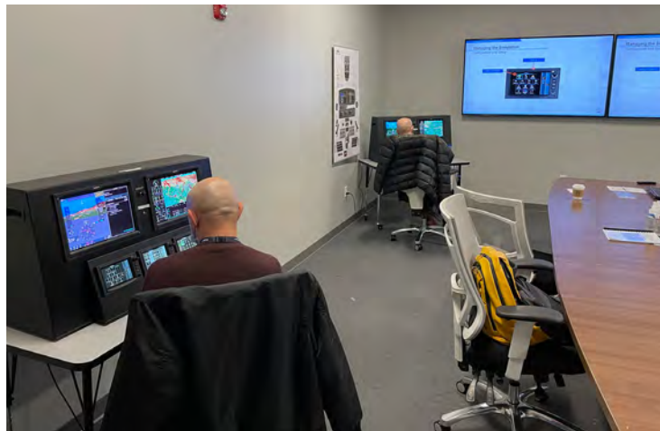
Above Garmin G3000 desktop trainers helping pilots to master the avionics and flightdeck on the first day
