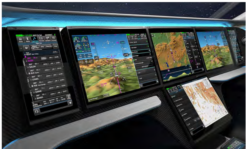
Above Honeywell's new Anthem flightdeck can be huge like this for a business jet, or scaled down for smaller aircraft
