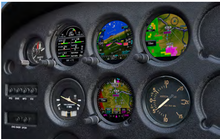
Above Garmin's GI 275 is a round electronic flight instrument that's available in a number of different variants, including attitude indicator, attitude-direction indicator (ADI), course deviation indicator (CDI), horizontal situation indicator (HSI), multi-function display (MFD), and engine indication system (EIS)
