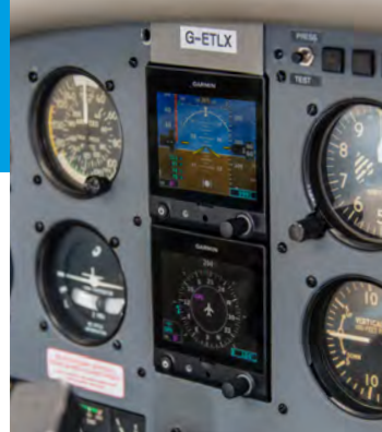
Left Garmin G5 twin stack set-up for attitude and DI Below uAvionix AV20 (left) and AV30 are available in certified and experimental versions
