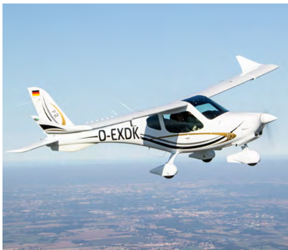
Above No struts! Below Centre tunnel adds rigidity to cabin Left Long narrow wings ('high aspect') are good for stability and endurance. Winglets reduce drag and improve wing performance further
