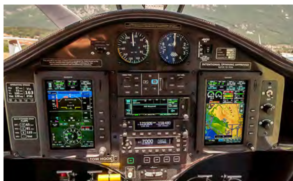
Above Dual Garmin G3X Touch screens are standard
