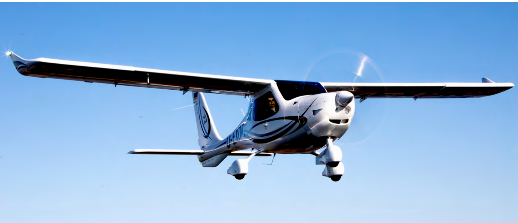
Above No struts! Below Centre tunnel adds rigidity to cabin Left Long narrow wings ('high aspect') are good for stability and endurance. Winglets reduce drag and improve wing performance further
