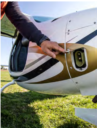
Above Garmin G3X flight-deck with 3D views on the display Right Fixed portion of the tailplane - the so-called 'beaver tail' - helps pitch stability Below Clean finish to airframe Left External power socket just one of many features on F2. Useful when ground training on the G3X panel with the engine off
