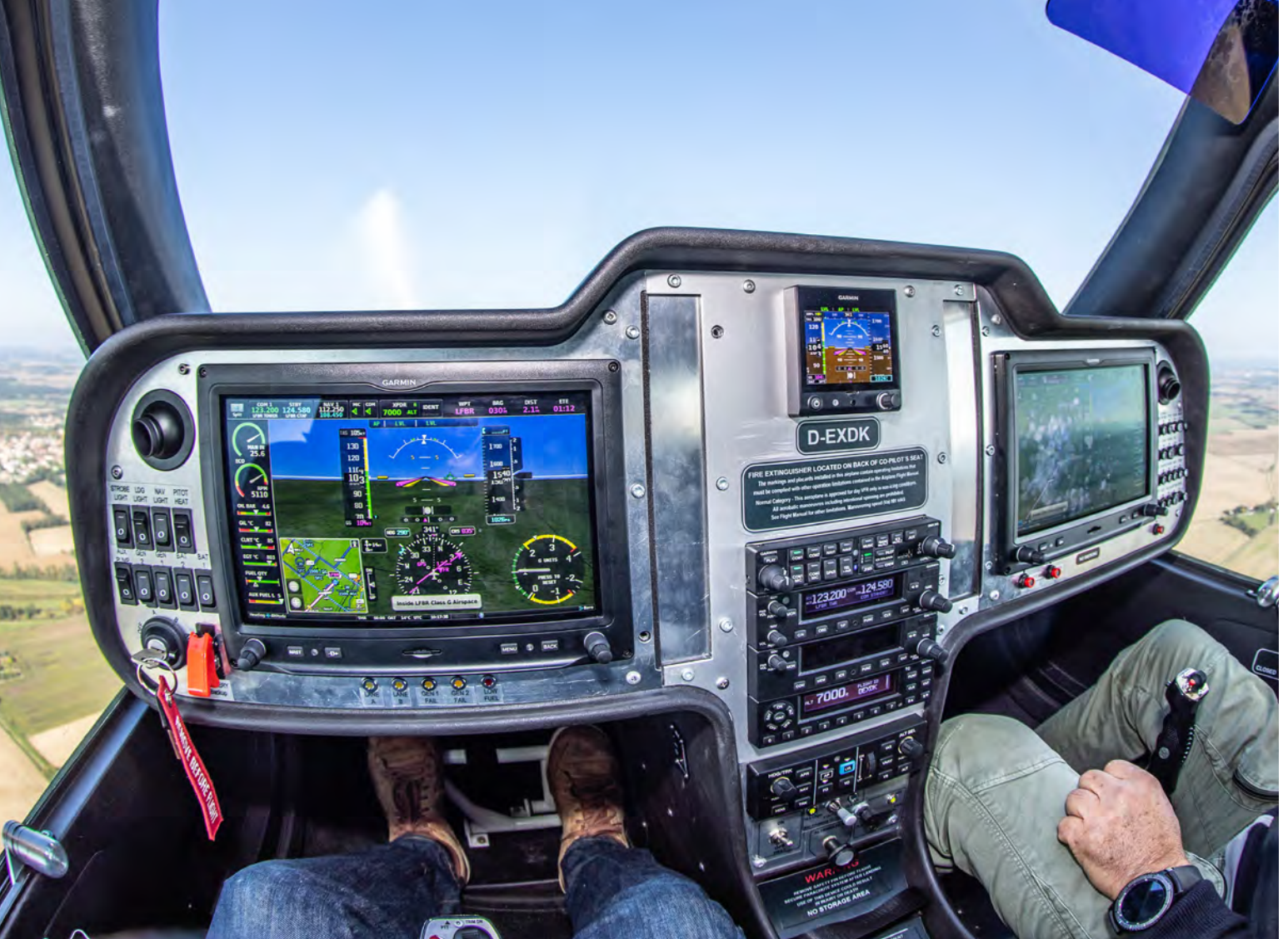
Above Garmin G3X flight-deck with 3D views on the display Right Fixed portion of the tailplane - the so-called 'beaver tail' - helps pitch stability Below Clean finish to airframe Left External power socket just one of many features on F2. Useful when ground training on the G3X panel with the engine off
