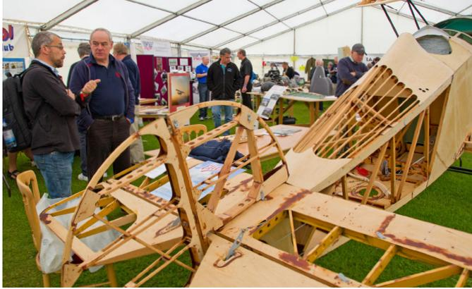
**Above** Building with wood means assembling parts, which then glue together to make an airframe
