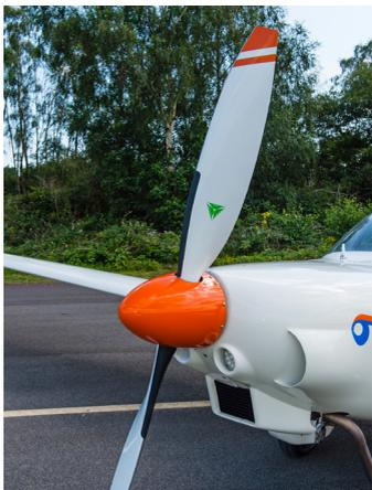
**Above** The Rotax sits further forward than the original Grob engine and is enclosed under a new, vertically split, cowling
