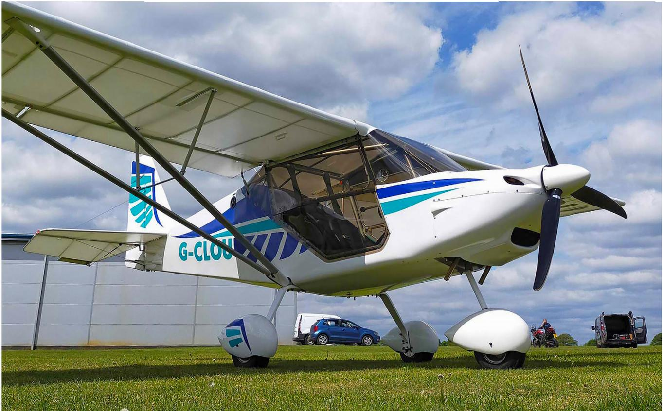
Can existing microlights have their max weight raised to 600kg? Yes, so long as they are proved to be technically capable of meeting the design requirements at the higher weight – which may mean modifications. The Skyranger Nynja, pictured, is one such aircraft.
