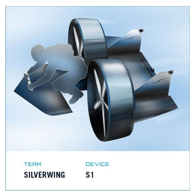
**Team's Device Description:** This device is a canard-wing configuration around a person in motorcycle-like orientation powered by two electric motors with ducted rotors. The aircraft makes a 90 degree transition from vertical take-off to horizontal cruise flight.
