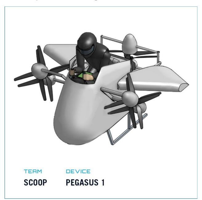
**Team's Device Description:** The Pegasus is a Y6 tilt rotor with a wing and a hybrid powertrain with a cruise speed of 70 knots.
