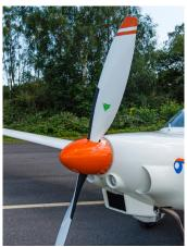
**Above** The Rotax sits further forward than the original Grob engine and is enclosed under a new, vertically split, cowling **Right** You can spec your Grob Able with the basics, or you can add Garmin's G3X and more
