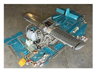
**Above** Rivet together the parts shown here, add an engine, propeller and instruments, and you'll have a Van's Aircraft RV-14 like the one shown top right, on the opposite page
