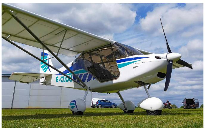
Can existing microlights have their max weight raised to 600kg? Yes, so long as they are proved to be technically capable of meeting the design requirements at the higher weight - which may mean modifications. The Skyranger Nynja, pictured, is one such aircraft.
