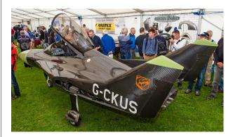
Above How about building your own single-seat jet, powered by four mini-turbine engines? This amazing machine, the Conway Viper designed and built by Barry Conway shows just how much you can do within the allowances for the SSDR (Single-seat deregulated category).
