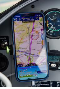
Far left New PowerFLARM Fusion box is a startling shade of orange, but otherwise identical form factor and mounting points Left Green circle is a Mode-S indication from the Fusion unit showing on an iPhone running SkyDemon
