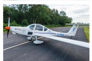
Above See what I mean about those long wings and the big tail? Left It is possible to take the wings off the Grob, but they're pretty much exclusively stored with the wings on. It is impossible to close the hatch if not correctly rigged Below left For nosewheel power pilots, steering on the ground and minding those long and relatively heavy wings can be a bit of a learning curve Below Airbrakes can be locked into the half-way position with the aid of that retractable nylon
