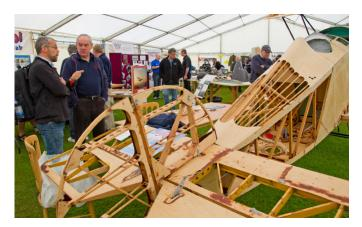
wood means assembling parts, which then glue together to make an airframe Left Tube and fabric is a time-honoured. but effective, way to build an airframe. This is a KEA Safari **Below** Composite kit aircraft are usually assembled from multiple premoulded parts **Bottom** Aluminium
